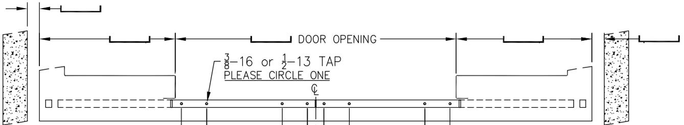
G.A.L. STANDARD SHEAVE MOUNTING HOLES ARE  $4\frac{1}{8}$   $\phi$  WITH  $\frac{3}{8}$  BOLTS.
