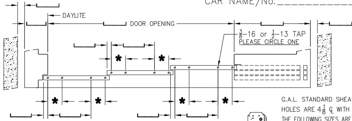
G.A.L. STANDARD SHEAVE MOUNTING HOLES ARE  $4\frac{1}{8}$   $\phi$  WITH  $\frac{3}{8}$  BOLTS.
