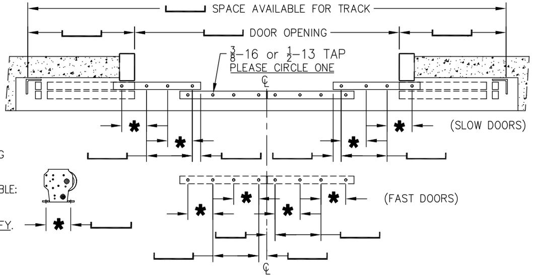
G.A.L. STANDARD SHEAVE MOUNTING HOLES ARE  $4\frac{1}{8}$   $\phi$  WITH  $\frac{3}{8}$  BOLTS.
