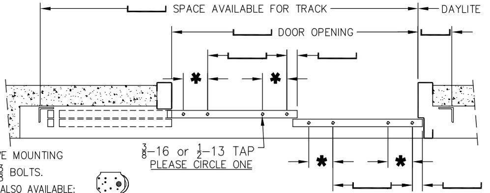
G.A.L. STANDARD SHEAVE MOUNTING HOLES ARE  $4\frac{1}{8}$   $\phi$  WITH  $\frac{3}{8}$  BOLTS. THE FOLLOWING SIZES ARE ALSO AVAILABLE:  $(3\frac{3}{4})(4)(4\frac{1}{4})(4\frac{1}{2})(4\frac{5}{8})(4\frac{3}{4})$  IF OTHER DIMENSION PLEASE SPECIFY.
