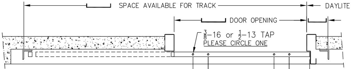
G.A.L. STANDARD SHEAVE MOUNTING HOLES ARE  $4\frac{1}{8}$   $\phi$  WITH  $\frac{3}{8}$  BOLTS.
